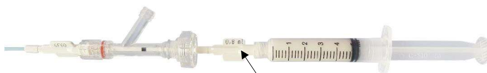
Fig. 11. Dead space volume of the catheter
