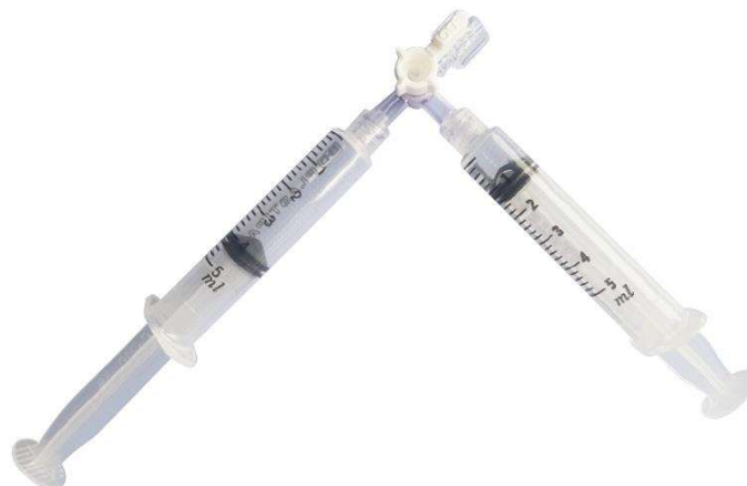
Fig. 10. Syringes connected with a three-way stopcock
